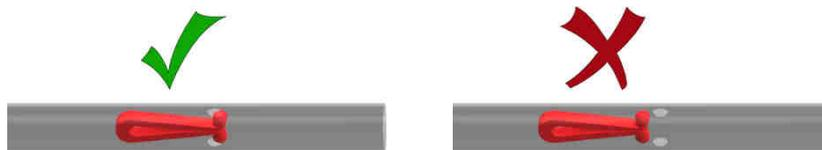
5. Use a screw driver to carefully move the red spring into position and make it snap out thru the spring holes on both sides.
